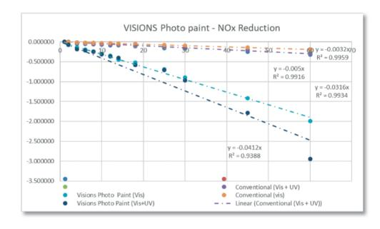
By activating the photocatalytic building material (turn on the light) the pollution level in the 'Green House' was reduced up to 61.7% while in the conventional one up to 24.6%. All side effects (adsorption on walls, photolysis, photocatalysis etc) was also estimated.
